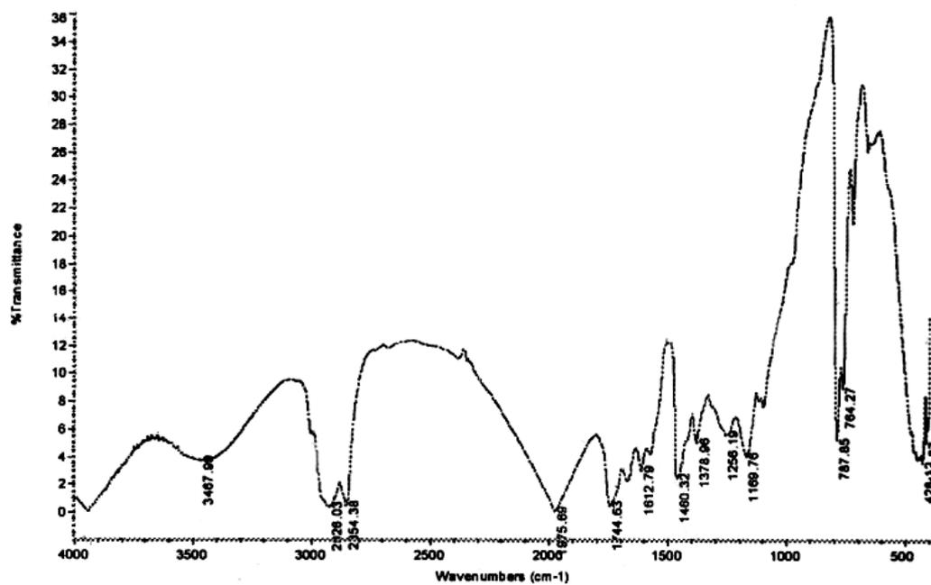
Fig.3 : infrared spectra for compounds separated from virgin Iraqi olive oil by irradiated natural silica using ethanol as solvent (irradiation time 1/2 h).
