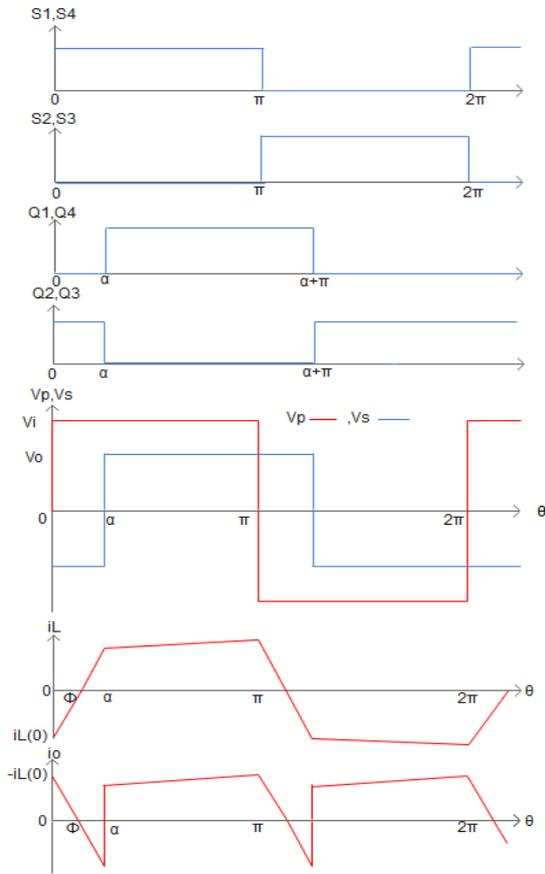
Fig. 6 Switch operation pulses and voltage and current waves of the dual active bridge in forward mode condition
