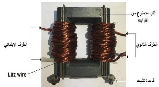
Fig. 9 the practical model of the designed high-frequency transformer
