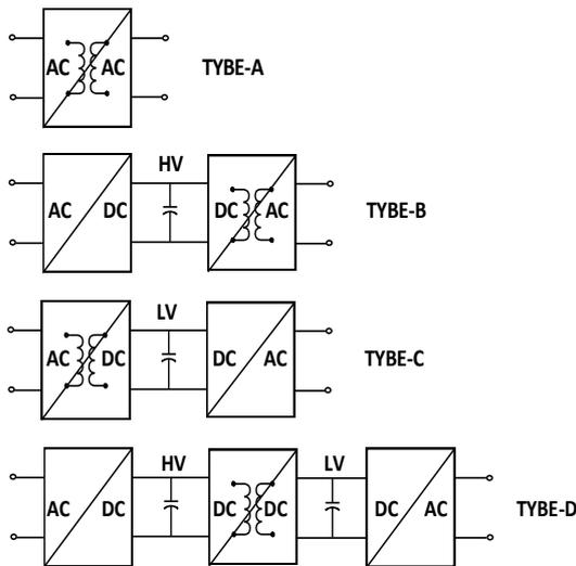
Fig. 2 Topography classification of solid state transformers.
