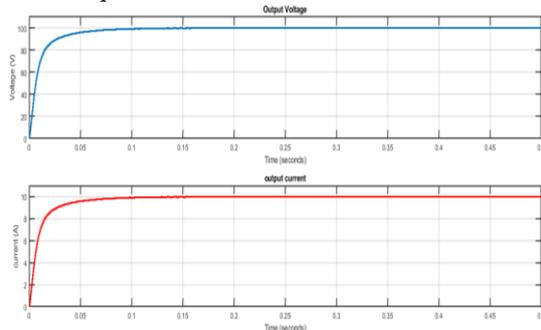
Fig. 14 Output voltage and output current for SAB
