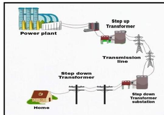
Fig. 1 Components of an electrical power system
