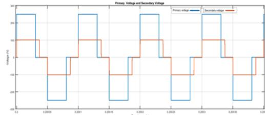
Fig. 11 Primary voltage ( $V_p$ ) and secondary voltage ( $V_s$ ) of a high frequency transformer
