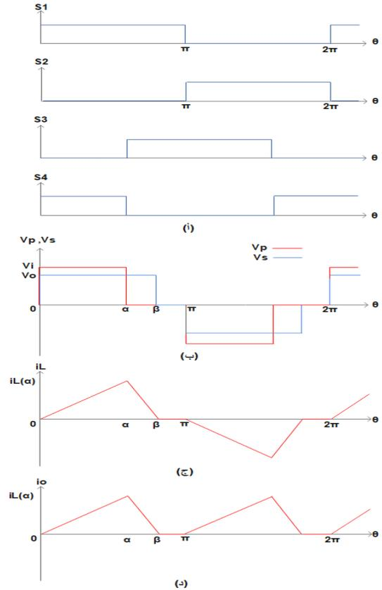
Fig. 5 Switch operation pulses and voltage and current waves of the single active bridge in discontinuous conduction mode
