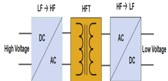
Fig. 7 DC-DC converter with high frequency transformer
